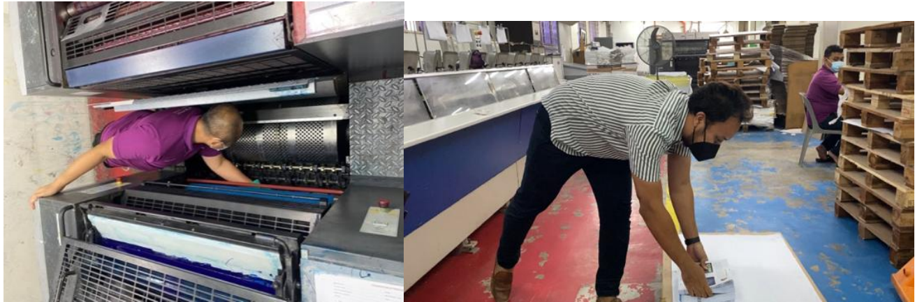
Figure 7: Operator adopting an awkward posture while accessing internal machine components and during paper handling, UiTM Shah Alam.
